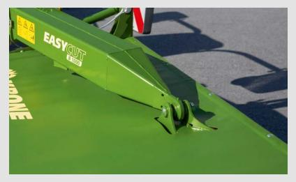
The mower is mounted on a pin which pivots in a ball bearing at the end of the outrigger arm. This design provides plenty of movement and exemplary contouring. In addition, the headstock features a standard and integral breakback system for effective impact protection.
